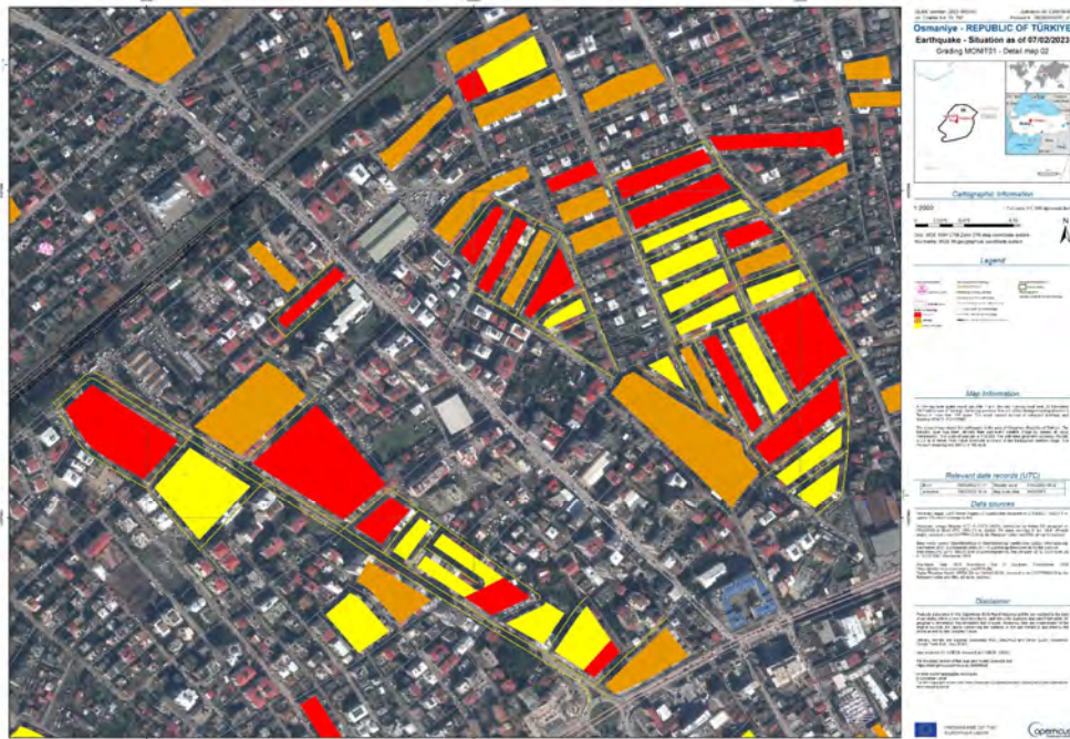
Figure 14: Damage grading in Osmaniye (Source: Copernicus EMS) https://emergency.copernicus.eu/mapping/ems-product-component/EMSR648_AOI06_GRA_MONIT01_r1_RTP02/1
