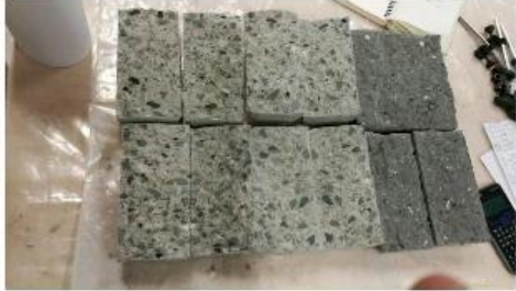
Fig.4: Splitting Tensile Strength Cylinders after testing
